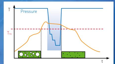
Void-free soldering with lead-free solders is an important prerequisite for the production of power electronics. However, minimal void rates are only possible with soldering processes which subject the molten solder to a vacuum, making it easier for any remaining residues to escape from the solder joints. For this reason, the Condensio can be equipped with a vacuum pump upon request. This results in solder joints with surface contact ratios of greater than 99% in many cases.
