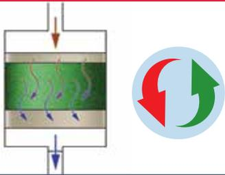
A partial vacuum is generated when the vapour is drawn off, assuring quick drying of the PCBs. The vapour is cooled down after it has been drawn off. After it has condensed, it is filtered and impurities are removed. The fluid is then returned to the soldering process. Due to the fact that the process chamber is hermetically sealed, only minimal loss results from vaporization during the soldering process. Medium consumption, as well as costs, are thus significantly reduced.
