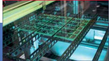
The assemblies are transported strictly horizontally through the soldering system. Furthermore, the PCB is stationary during the soldering process. In this way, components cannot be shifted out of place while the solder is molten. It has thus been possible to eliminate a considerable disadvantage associated with conventional vapour phase soldering systems within which continuous vertical motion of the PCBs is required during soldering. Scrap rates are reduced as a result, as well as costs.
