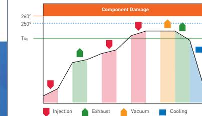
A defined quantity of an inert fluid (usually perfluoropolyether) is vaporized during reflow soldering in the process chamber, which is hermetically sealed by means of a bulkhead. The vapor allows for extremely effective heat transfer to the PCBs due to the release of heat during condensation, and the temperature of the medium remains constant. In addition to this, the medium's boiling point limits the
