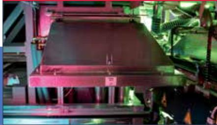
After the soldering process, the PCB can then be advanced out of the process chamber for cooling. Here you're provided with the option of reducing the standard air cooling temperature to a constant low level with the help of water. This makes it possible to cool the PCB absolutely uniformly, and above all more quickly. Furthermore, the machine's ambient temperature is not significantly increased
